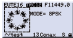
Constell. DVB-S2 = 8PSK, T = COFDM, C = QAM and modulation parameters
